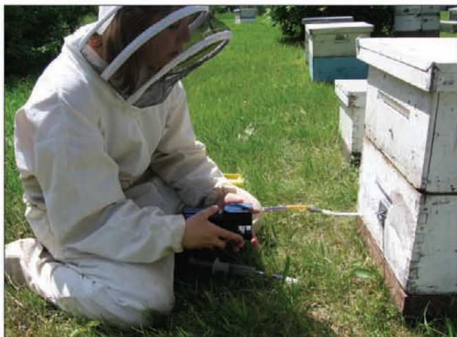
University of Manitoba researcher measures formic acid concentrations in colonies treated for Varroa mites.
