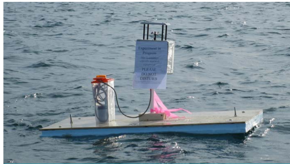
Rotorod® pollen collecting device floating on Lake Clearwater (photo by G. MacInnis)
